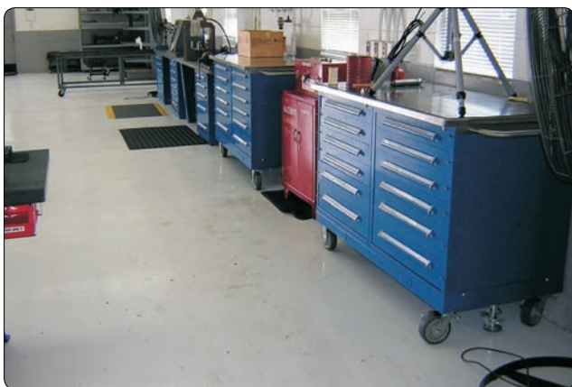
Mobile workcenters can be easily moved and configured to create a custom designed work area.
